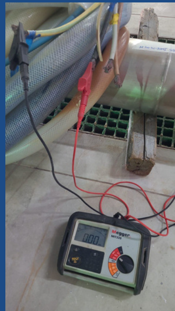
FIGURE 2 - PUMP DETAILED INSPECTION: A) PUMP BEING REMOVED FOR DETAILED INSPECTION B) INSULATION RESISTANCE TEST SHOWING 0 MOHM
